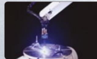
Tracking sensor for TIG welding
