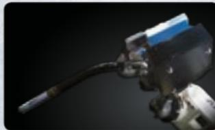
Laser start point detection sensor
