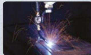
Tracking sensor for MIG/MAG welding
