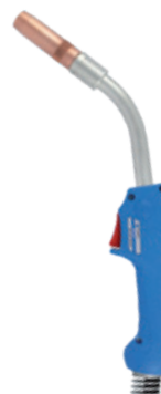
TBi 6G 60% (10 min.) Mix: 350 A CO 2 : 380 A Ø 1.0-1.6 mm
