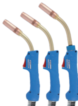
TBi 7G (S, L, DR) 60% (10 min.) Mix: 310 A (S: 230 A, DR: 220 A) CO 2 : 330 A (S: 250 A, DR: 250 A) Ø 1.0-1.6 mm
