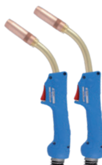
TBi 7W (S, L) 100% (10 min.) Mix: 450 A (S: 400 A) CO 2 : 500 A (S: 450 A) Ø 1.0-1.6 mm
